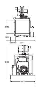
Drawings based on standard open power 480 volt standby generator. Lengths may vary with other voltages. Subject to change without notice. Sound data as measured at 23 feet (7 meters) in accordance with ISO 8528-10 at standby rating.
